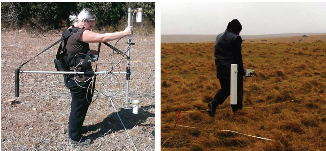
FIGURE 2B. LEFT: PAIR OF GEONICS G-858 CESIUM VAPOUR MAGNETOMETERS SET UP AS A 1m VERTICAL GRADIOMETER. RIGHT: GEOSCAN RESEARCH FM256 0.5m SENSOR SEPARATION FLUXGATE GRADIOMETER (CAN ALSO BE MOUNTED ON A FRAME WITH A SECOND INSTRUMENT, WITH A 1m TRAVERSE INTERVAL) FOR HANDHELD SURVEYS.
