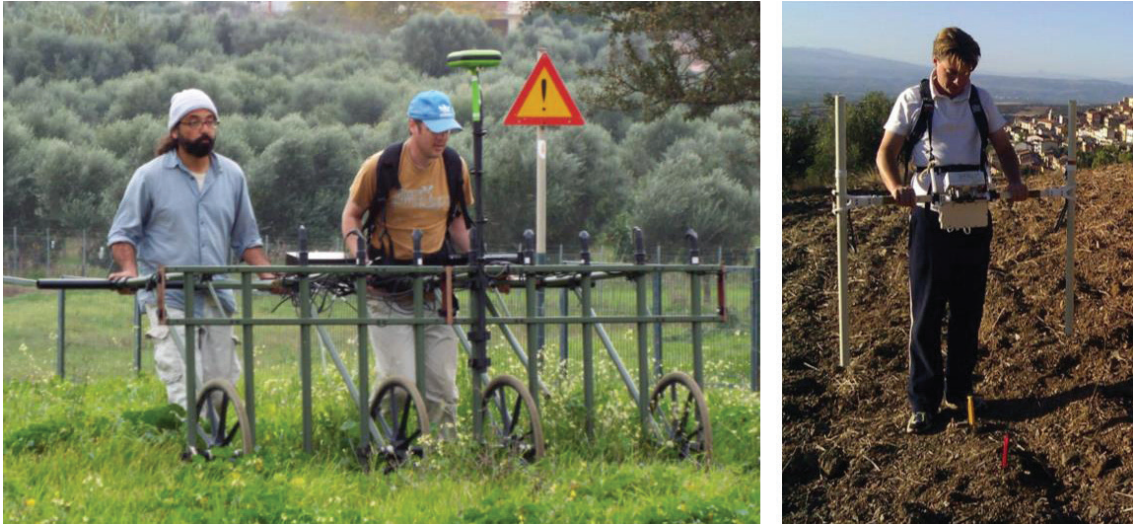
FIGURE 2A. LEFT: A SENSYS 8 FLUXGATE GRADIOMETER ARRAY CART SYSTEM, NAVIGATED BY DGPS (SEE BELOW), AND SET UP WITH A 4m SURVEY SWATH, WITH 0.25m TRAVERSE SEPARATION. RIGHT: BARTINGTON DUALGRAD 601, 1m SENSOR SEPARATION FLUXGATE GRADIOMETER WITH 1m TRAVERSE INTERVAL FOR HAND HELD SURVEYS
