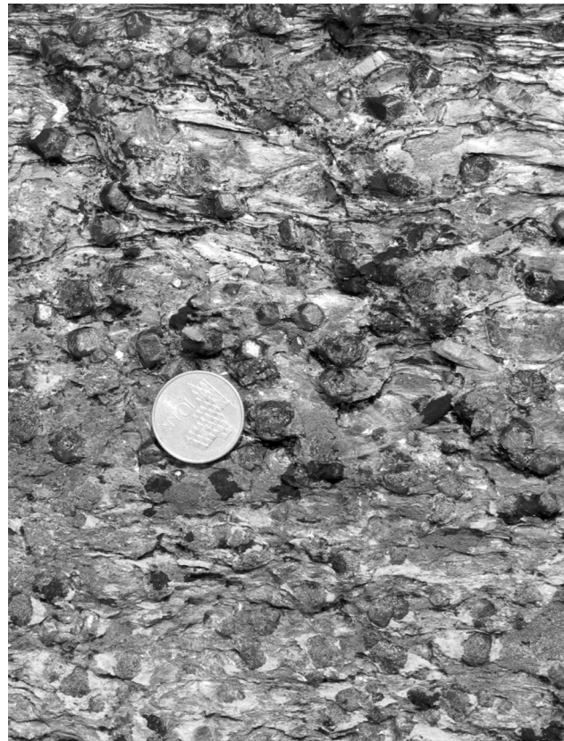
FIGURE 1.2: THE GARNET MICA SCHIST FROM HYLLESTAD. THE DARK-RED GARNETS SEEN ARE C. 2-5MM IN SIZE (PHOTO: ØYSTEIN J. JANSEN)
