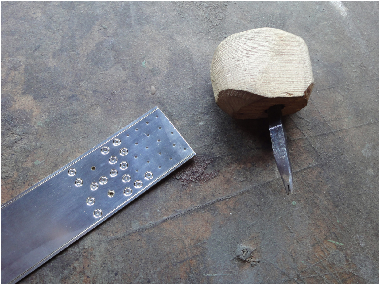
Figure 5: Experimenting with methods and techniques of tinning and ring-and-dot decoration to match those found on the archaeological examples at Cumwhitton (Photograph: Adam Parsons)
