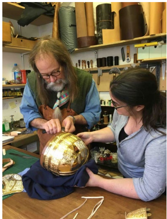
Figure 12 (above): Helmets under construction in the lab (© Drakon Heritage and Conservation)
