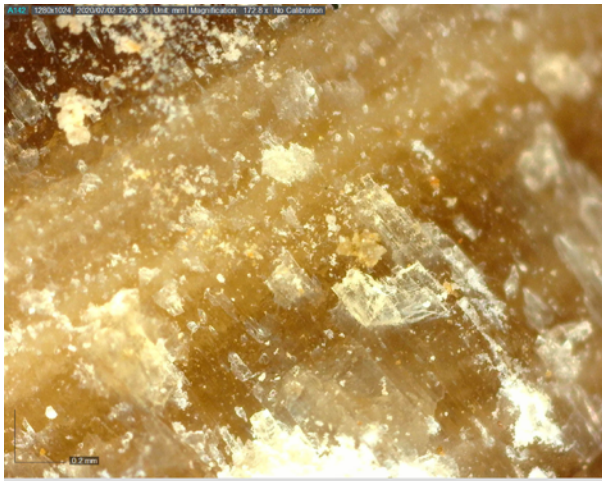
Figure 13: Solunt. Detailed digital microscope view of the calcitic laminations of the SOL 18/10 sample within substratum fracturing (photo: V. Ollivier).
