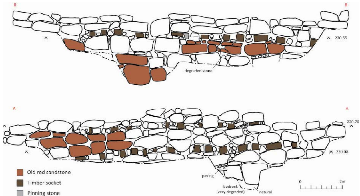
Figure 3.65: Elevations of the external (above) and internal (below) faces of Wall E in Trench A, detailing the use of Old Red Sandstone, the timber sockets and the bedrock foundation.
