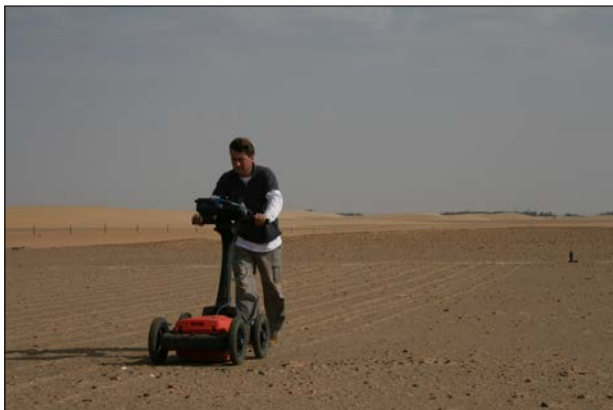
Plate 14.1. GPR survey at Kawa (photo: S. Hay).
