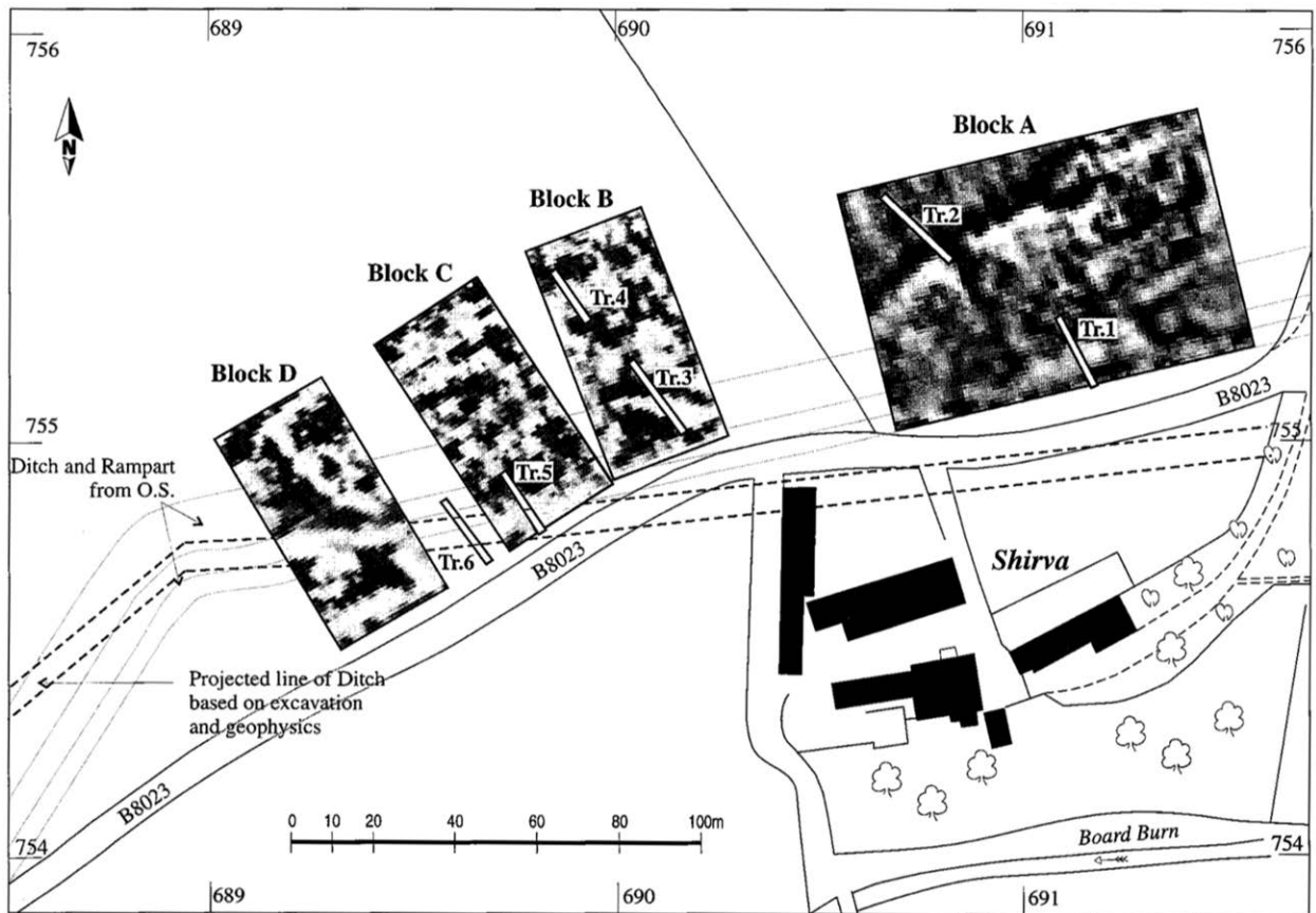
Figure 4.2.7. CFA resistance survey at Shirva, Blocks A-D, showing high (dark) and low (light) resistance values (after Glendinning 1998a, Fig. 2).
