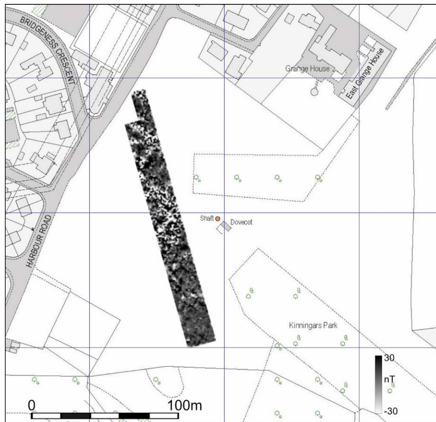
Figure 7.5.2. Gradiometer survey transect across Kinningars Park.
