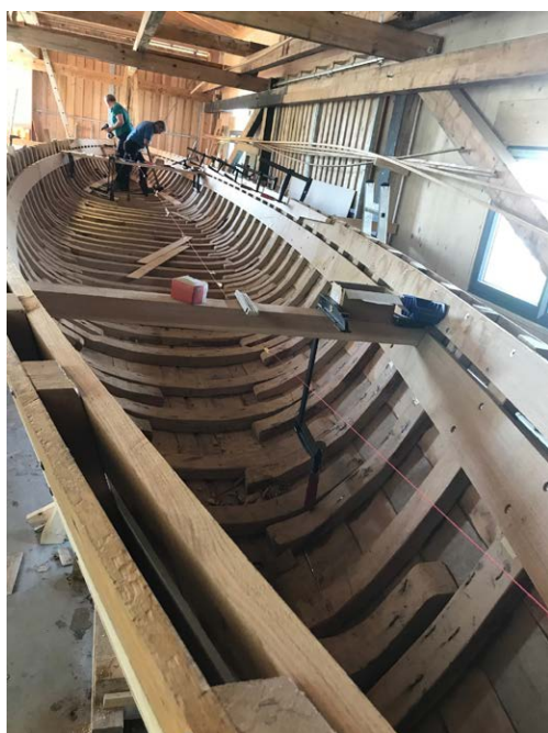
Figure 165. Building the The 'Danuvia Alacris' replica ship which rowed down the Danube in 2022
